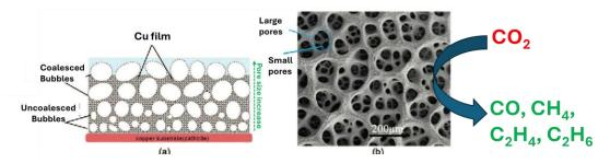
**Fig.1**: Schematic representation of the DHBT method for synthesizing Cu foams (a), and an SEM image of a Cu-foam sample produced via the DHBT approach (b).
